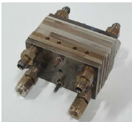
Fig. 7. Methanol fuel processor B integrated with fuel vaporizer, heat exchanger, methanol steam reformer and catalytic combustor.
